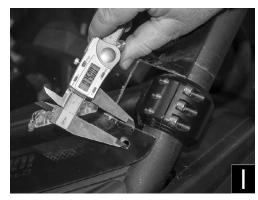
Step 13: Measure 1" in from outside edge of the windshield as shown in Figure J.
