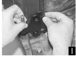
**Step 11:** Align the top slot of the Upper Hinge Bracket - Driver [P5] to the upper hole and then loosely install the self-tapping screw [P12] with washer [P11]. Make sure to leave 1/2" gap. When done, make sure the bracket is vertically straight and then loosely install self-tapping screw [P12] with washer [P11] to the bottom slot into the plastic and frame (Figure J).
