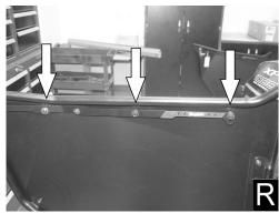
**Step 20:** Repeat instructions for Door Assembly - Passenger Side [P2] with the appropriate passenger side hardware (Figure S).
