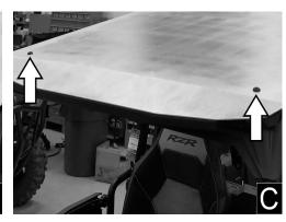
**Step 5:** Carefully place and align Rear Roof Panel [P2] to the Front Roof Panel. Install panels together using hardware: insert bolt [P5] through nylon washer [P6] and rubber washer [P7] and then install through the panels where shown (Figure D). Hand-tighten using locknut [P8].
