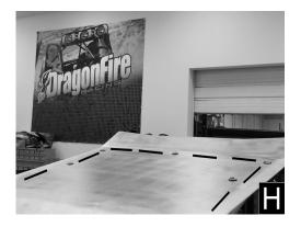
Step 11: Tighten all hardware until roof is secured. Do not overtighten hardware; overtightening will cause dimples.
