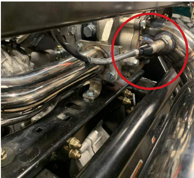
22. Install Dynojet AFR sensor into turbo exhaust. Run wires along right side of vehicle into the front cab area of the machine. Take care not to pinch or install the wire where damage can occur. Plug color matched wires into AFR Module
