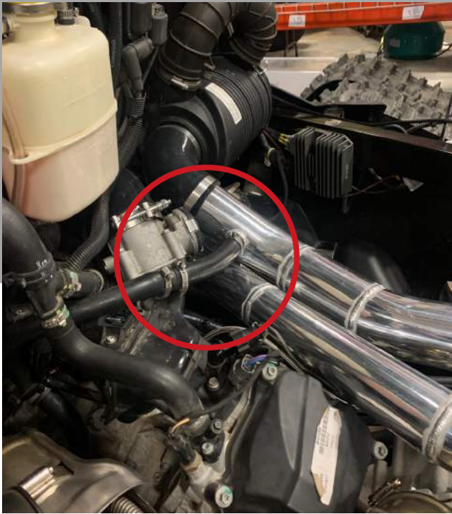
20. Connect crank case breather line to 3" turbo cold air intake
