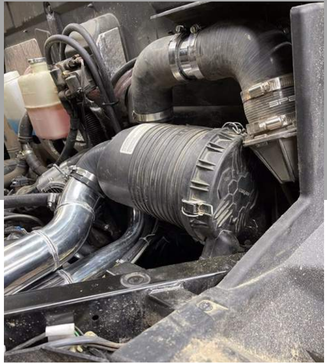
21. Install U bend silicone fitting assembly to top of the air filter box. Tighten down clamp
