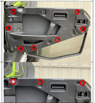
10) Uninstall the 3 fasteners at top edge on the inside of the lower door.
