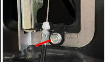
25) Mount the Z end of the cable through the hole on the Latch Lever and snap the ring on the end cap casing into the Latch Cable Standoff.
