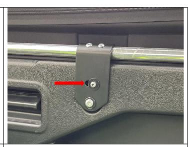
32) The 3<sup>rd</sup> Tab on the Front Shroud (Step 5) will use the screw from the roof to be fastened to the vehicle.
