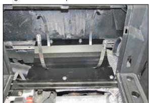
11. Install the filter base plate assembly as shown using the provided hardware.
