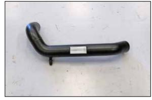
21. Install the provided vent fitting into the  $K\&N^{\circledast}$  intake tube.
