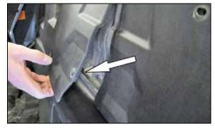
3. Pull back the inner lower corners of the back panels to gain access and remove the two air filter housing mounting bolts.
