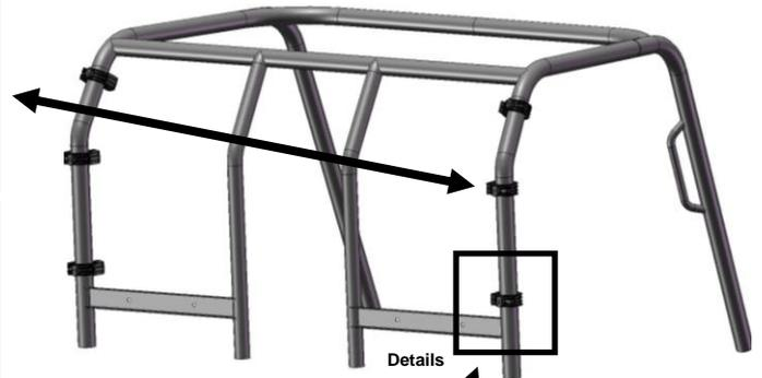
To apply more or less tension to the roll cage, simply rotate the clamp handle from the tension screw as shown below. Over tightening clamps to roll-cage could cause parts failures.
