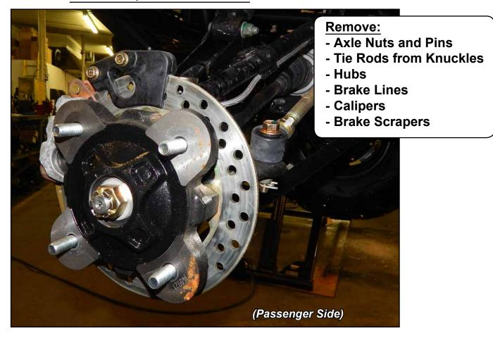
Rear Components Removal: Keep all components removed from machine.
