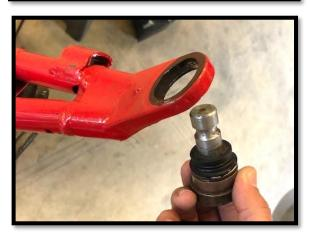
8. Before pressing the ball joints into the new High Lifter control arms, you may need to remove any built-up powder coating that could prevent the ball joint from seating all the way.
