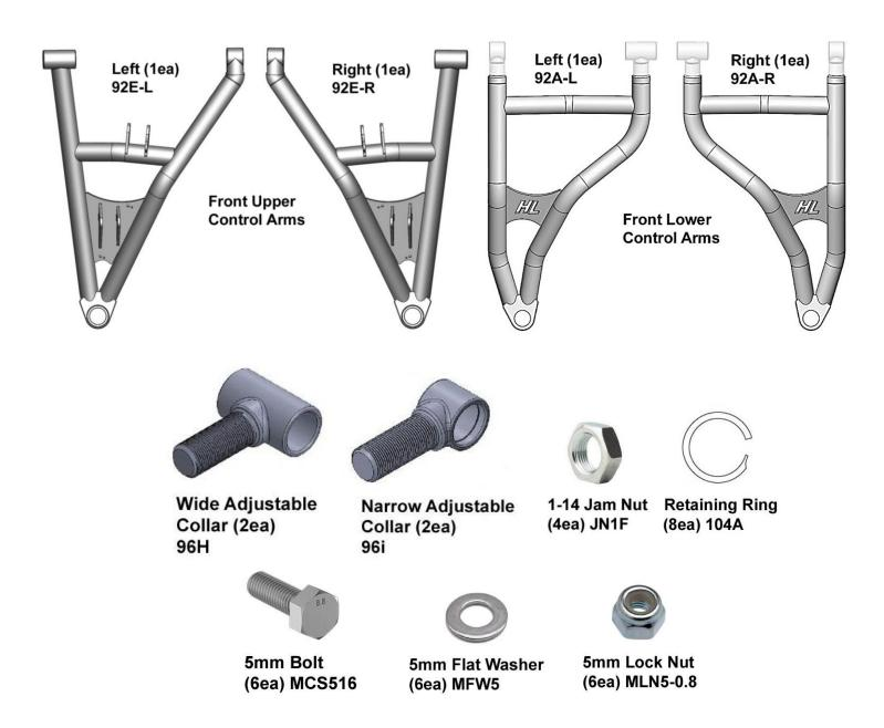
NOTE: These instructions are used in kits that come <u>with</u> or <u>without</u> ball joints. If you have purchased a kit that has the ball joints preinstalled, then the ball joints are not shown in parts diagram.
