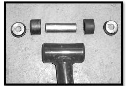
11. In the next steps, reinstall the bushings and sleeves into the new arms and adjustable collars. If you place some grease on them, it makes the installations easier.
