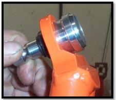
3. When pressing in the ball joint, support the ball joint end of the arm in a press with something solid below the arm and will allow the end of the ball joint to pass through completely. Be sure the support arm properly to allow the ball joint to pass through the hole straight and without interference. Again, be sure the boot will clear the fixture you are pressing into and the hole is deep enough for the full length of the ball joint to press into the arm.
