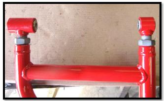
13. The new lower High Lifter control arms will <u>already come adjusted to factory length</u>. If you need to readjust the collars, place the arms on a flat surface. Measure from eyelet to ball joint on the factory arm, and then set adjust the new arm to those lengths.
