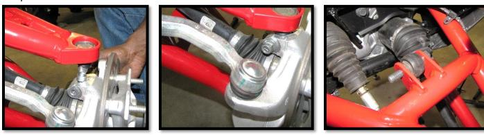
16. If you have not already done so, reconnect the bottom of the shock to the upper arm using the stock hardware. Fasten to factory specifications.
