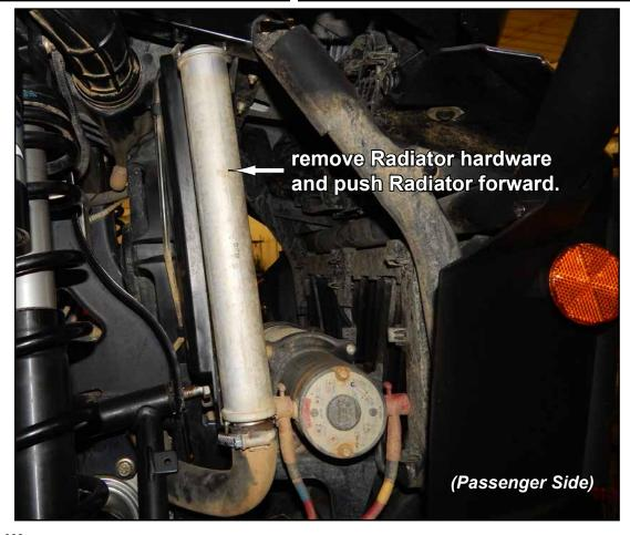
Removal: Keep all components removed from machine.
