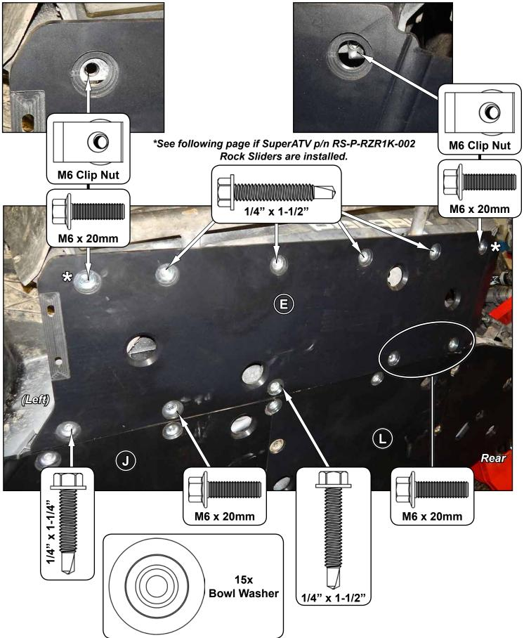
Use hardware shown if SuperATV p/n RS-P-RZR1K-002 Rock Sliders are installed.
