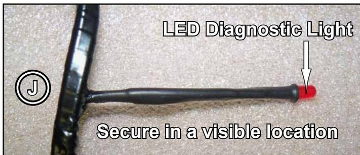
When activated, LED Diagnostic Light will flash once for about 1 second before turning off indicating proper function. Should different patterns occur, contact SuperATV.
