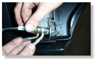
Disconnect the banjo bolt and brake lines from the master cylinder.
