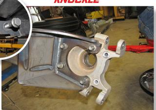
Secure the knuckle to the trailing arm by using the factory (4) nuts & (4) washers (17mm) USE TOE SHIMS HERE TO MAKE CAMBER CORRECTIONS.
