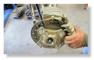
Re-secure fitting to caliper if you have not done so already. Connect the caliper to the hub assembly. (15mm)
