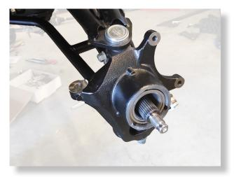
Remove the cotter pin, axle nut, and washers from the hub assembly, then remove the hub. (27mm) KEEP FACTORY HARDWARE. 4
