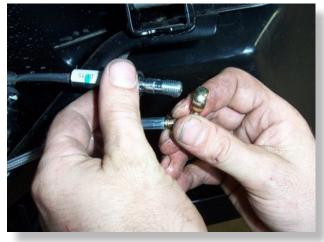
Install the new **57**" **FRONT (PA) brake line** to the banjo bolt. Run the line back through the frame and to the **RIGHT (PA) side hub.**
