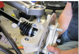
Slide the axle through the hub assembly. Connect the lower arm at the knuckle, then the upper arm. Secure with factory hardware.
