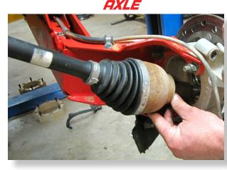
Completely romove the axle by removing it from the knuckle and the differential.
