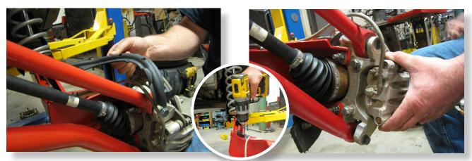
Remove the brake line guard by removing the bolts securing it.
