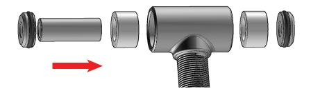
Once the bushing is inserted, use a socket, of the same diameter as the bushing to press it in all the way.
