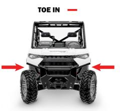
If the FRONT OF THE WHEELS are facing IN, adjust the tie rods IN or <u>REDUCE the length of the tie rod.</u>
