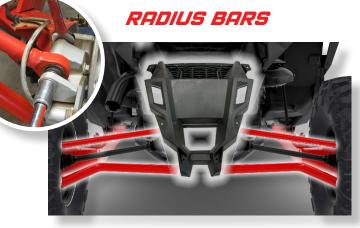
If you cannot access the radius bar mounting bolts due to the plastic bumper, remove it. Remove the nuts and bolts securing the UPPER & LOWER radius bars at the frame and hub.
