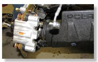
Disconnect the brake line from the caliper and upper control arm. Have a container ready to collect brake fluid.
