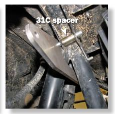
**Insert the (31C) spacer** between the original shock tabs. Run the bolt all the way through **DO NOT** secure hardware yet.
