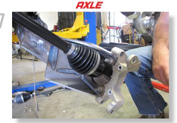
Install the new axle into the rear differential, then slide it into the knuckle.
