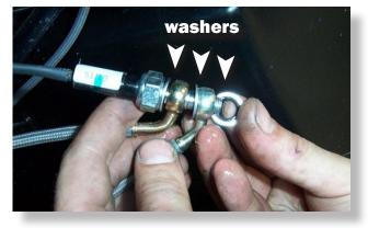
Save the factory washers that separate the two front lines. Remove the line from the UTV.
