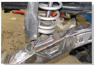
Secure the shock to the trailing arm using factory hardware.
