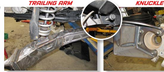
Install the new trailing arm to the frame, use factory hardware to secure.
