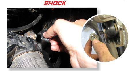
Once the arms are mounted, install the shock. Secure it with a M10x75mm bolt through the upper shock lift bracket, then install a 10mm washer and fasten with a 10mm lock nut.
