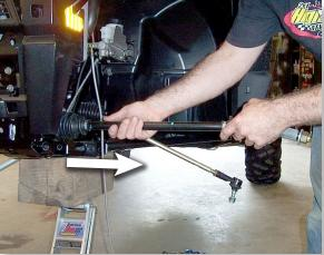
Remove the **Upper and Lower arms** by removing the **bolts** from the **frame. (18mm) Then remove the stock axle. KEEP ALL FACTORY HARDWARE.**
