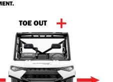
If the FRONT OF THE WHEELS are facing OUT, adjust the tie rods OUT or <u>INCREASE the length of the tie rod.</u>
