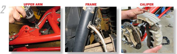
Remove the **brake lines** from arms and frame by drilling off the rivets. Remove the (2) **brake caliper mounting bolts (15mm) DO NOT disconnect lines from caliper.** Set brake caliper aside.
