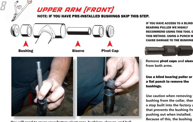
You will need to reuse your factory pivot caps, bushings, sleeves, and ball joints. Make sure that you inspect your bushings and ball joints for wear. Replace as needed.
