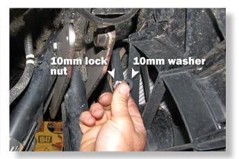
Secure the **bracket** in place with the **10mm flat** washer and **10mm lock nut.**
