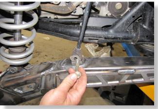
Secure the stability bar in place, use factory hardware.
