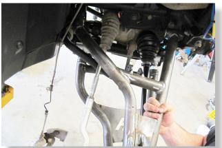
Using factory hardware, connect the new upper arm at the frame.
