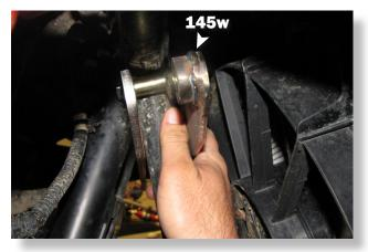
Install the **(145W)** bracket to the **FRONT** of the unit. (closest to the radiator)
