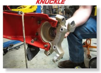
Remove the (4) nuts & washers that secure rear knuckle to the TRAILING ARM (17mm) Remove the rear knuckle. SET KNUCKLE ASIDE. KEEP FACTORY HARDWARE.
