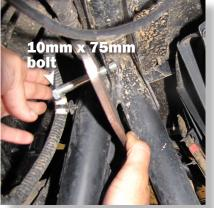
Insert the M10x75mm bolt through the bracket and tab.
