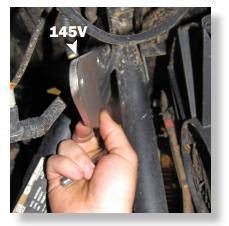
Install the (145V) bracket to the **REAR** of the original shock tab.
