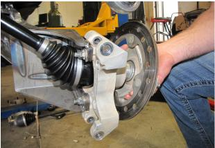
Slide the rotor on to the axle (make sure splines are lubricated with water resistant grease) Fasten using washers, castle nut, and cotter pin provided in the kit. (27mm)
