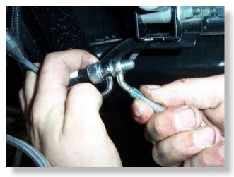
Install the new 40" FRONT (DR) brake line to the banjo bolt. Run the line back through the frame and to the LEFT (DR) side hub.
