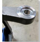
Once the bearing (31J) is in place, use a socket of the same diameter as the outer race to press it in all the way. Apply grease to outer race to ease install.
