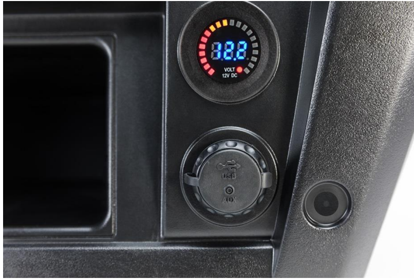
(FIG 10-2) Dual Accessory Mounted with after-market voltage meter mounted above
