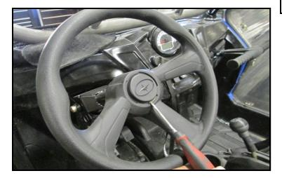
Fully remove the OEM steering wheel and replace it with the steering wheel hub adaptor. The hubs fits several models so the shaft might differ slightly from picture below. Then remove the center nut with a 24mm socket. To remove the wheel you will need to hit it slightly on the backside to break it free. If it does not come off then you might need to use a wheel puller to remove it.
