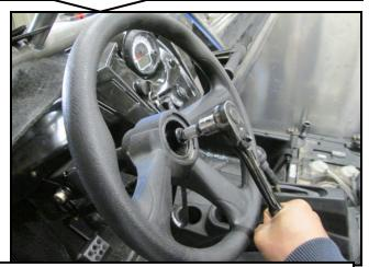
Make sure the hub is pressed as far as you can on to the tapered steering column by hand before putting washers in place. Make sure both washers are installed on the center of the shaft.
