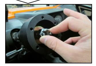
Place the wheel in the right location and tighten the hardware from your wheel down to the wheel manufacturer's specifications.
