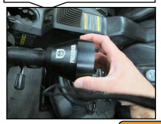
Re-install the factory nut on top of the 2 provided washers and tighten the nut to the vehicles manufacturers recommended torque specifications. Before final tightening, make sure the hub is aligned so the steering wheel is straight when driving straight.
