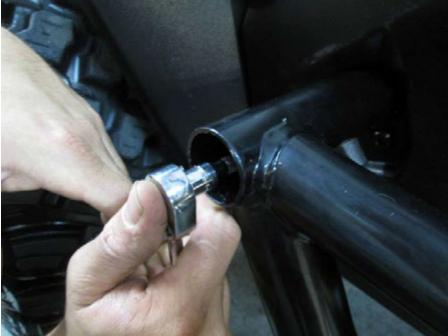
• Place the rock slider with the expansion anchors onto the vehicle. Make sure the sleeves of the expansion anchors are still seated properly in the grooves in the mounting holes of the rock slider before you proceed to tighten the anchors. Apply constant inward pressure on anchors as you tighten. It may be helpful for another person to hold the rock slider in place while you go around and evenly torque down the three anchors. DO NOT OVERTIGHTEN as you may shear the bolt in the expansion anchor.
