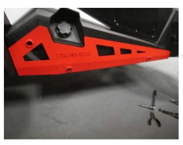
Adjust the placement of the rock slider to match the body lines as best as possible. Keep the rock slider snug up against the plastic as you go around and evenly torque down the three anchors. DO NOT OVERTIGHTEN as you may shear the bolt in the expansion anchor.
