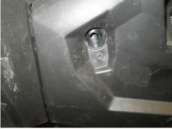
• Begin by removing any dirt/obstructions that may interfere with the installation of the rock slider. Make sure all of the mounting holes and surfaces are clear.
