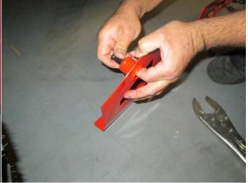
• Assemble the supplied expansion anchors [ITEM 1] with the rock slider as shown above. Insert the bolt, washer, and sleeve into the mounting hole first. The flat surfaces of the sleeve of the expansion anchor should fit into the groove in the mounting hole of the rock slider. Then, thread the nut on the back side, against the fingers of the sleeve. The flat surfaces of the nut should fit into the groove in the sleeve and create a snug fit.
