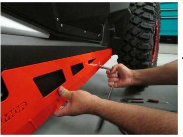
• Place the rock slider with the expansion anchors onto the vehicle. Make sure the sleeves of the expansion anchors are still seated properly in the grooves in the mounting holes of the rock slider before. Apply constant inward pressure on anchors as you tighten. It may be helpful for another person to hold the rock slider in place while you hand tighten the anchors. Do not fully tighten yet.
