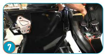
There is also adjustment in the latch plate assembly. You can adjust this with the 3 m6 bolts using a 4mm Allen wrench.
