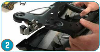
Pull the cover off the stock door by removing the 6 - t25 bolts.
