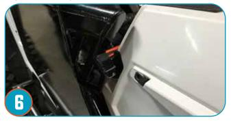
With the 3 bolts snug align the door so that it opens and closes smoothly. Make sure it latches. Then tighten the 3 t40 bolts.
