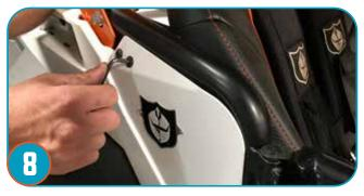
Next put on the quarter panel assembly with the hardware that came with your doors. (2 half clamps and 3 6mm bolts) Tighten with a 4mm Allen wrench.
