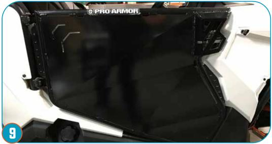
Now double check all hardware so that it is fastened tightly and correctly. Repeat these steps for opposite door.
