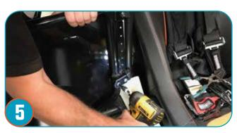
Install the new trail door on to the car with the 3 t40 bolts that you removed in the first step.
