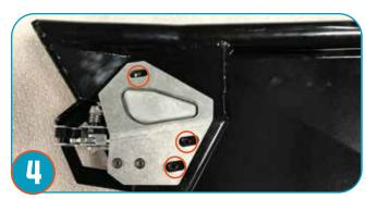
Install the paddle latch on your new Pro Armor trail doors using the provided latch plate with the t30 bolts that you removed from the previous step & 3-M6 bolts in hardware kit.
