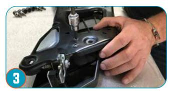
Remove the paddle latch from the door by removing the 2 - t30 bolts.
