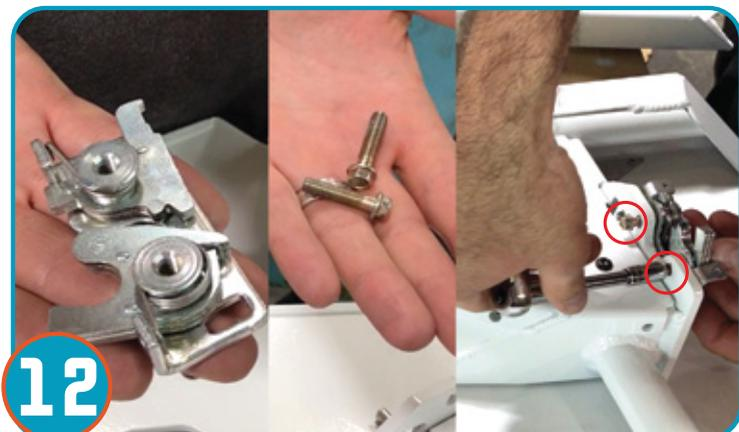
**12** Attach the slam latch to the door using 2 bolts removed from step 3. Only Thread half way. Repeat for opposite door.
