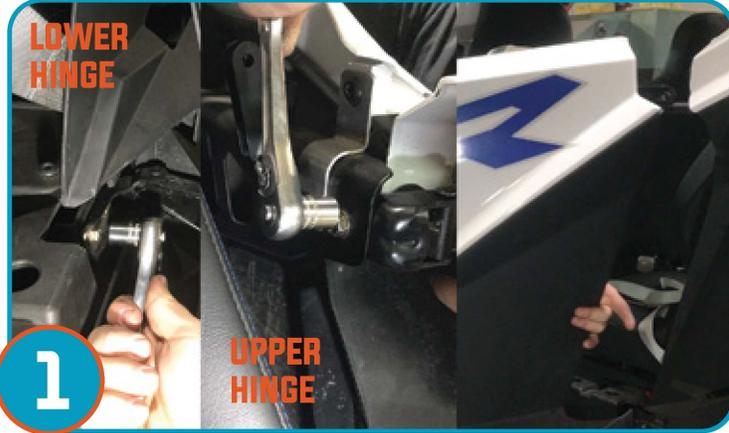
Remove stock rear door by removing 4 bolts per door and remove lower & upper hinge to remove door from vehicle. Repeat for opposite door. \*To allow for additional room to access hinge bolts un hinge or remove seats.
