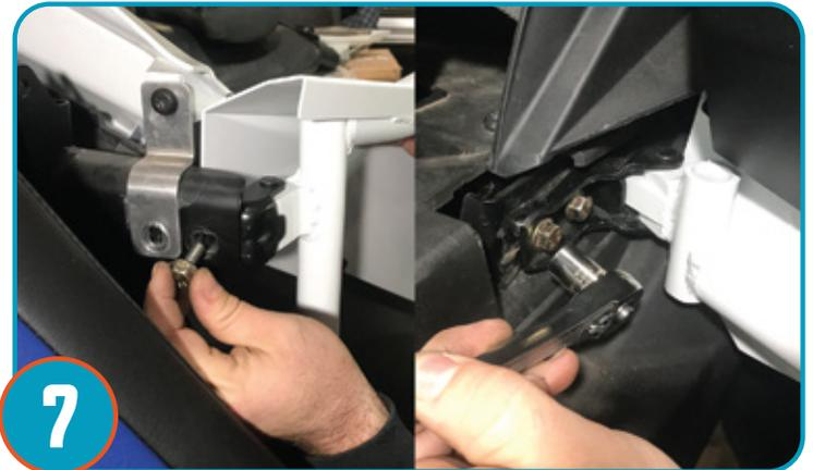
**7** Secure door with bolts provided (2) upper, (2) lower. Adjust door pitch as needed and torque to factory specs. Repeat for opposite door.
