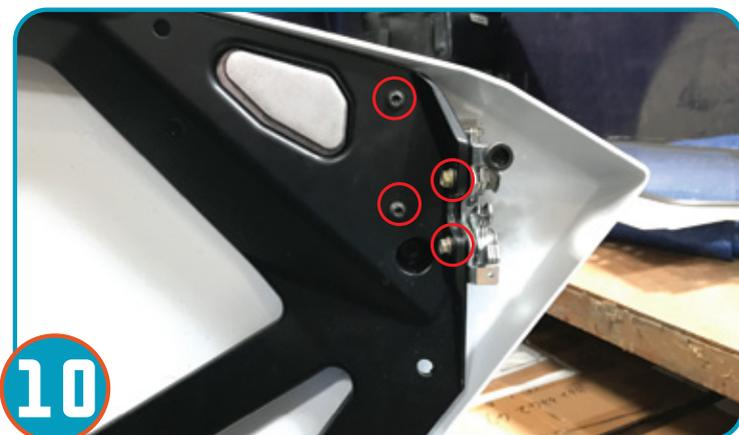
**10** Remove 4 bolts holding the OEM Paddle latch and slam latch on the stock door. Repeat for opposite side.
