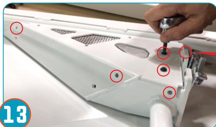
**13** Attach latch plate to door using (4) provided bolts. Secure all 8 bolts from steps 4-6.
