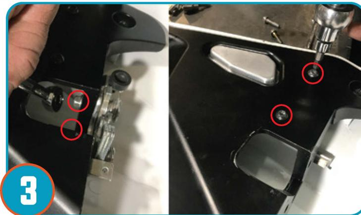
Remove four bolts holding OEM Paddle latch on the stock rear door. Repeat for opposite door.
