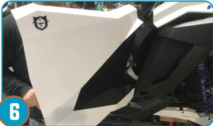
**6** Position door on vehicle lining up hinge bolt holes to door frame hinge. Use provided hardware to hold door in place.
