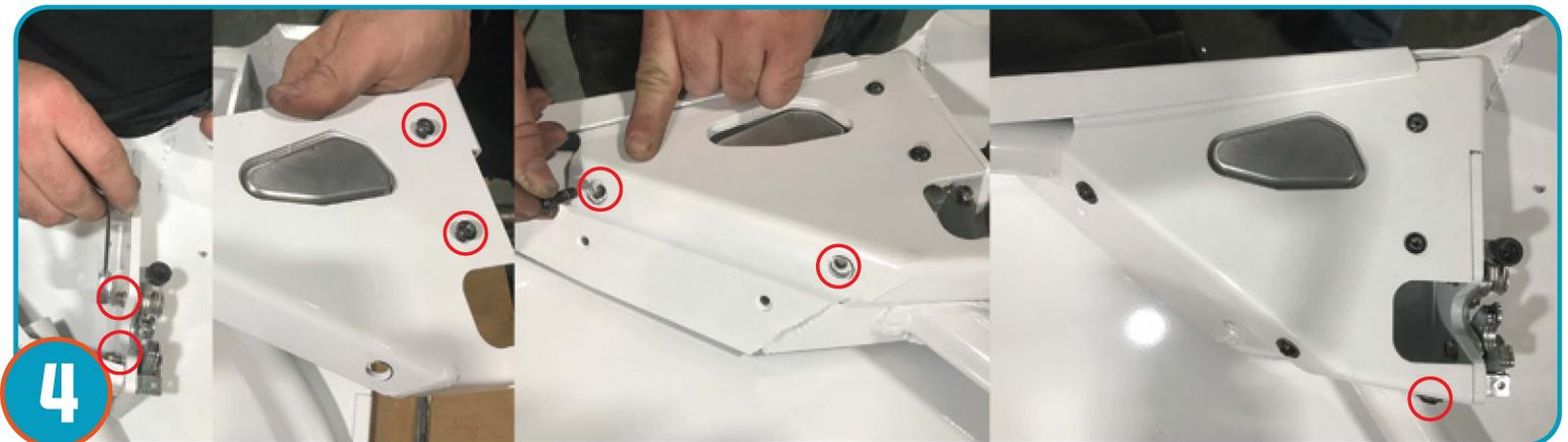
Attach the slam latch & paddle latch to latch plate (provided) as shown with the 4 bolts removed from step 3. Only thread half way. Attach latch plate to door using 4 provided bolts. Secure all 8 bolts.
