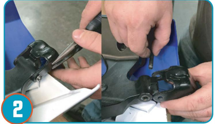
Stock hinges will be used for your Pro Armor door. Remove hinge by carefully removing the C-clip & sliding the pin from the hinge. Remove hinge from stock door. Remove bushings from door. Repeat for opposite door.
