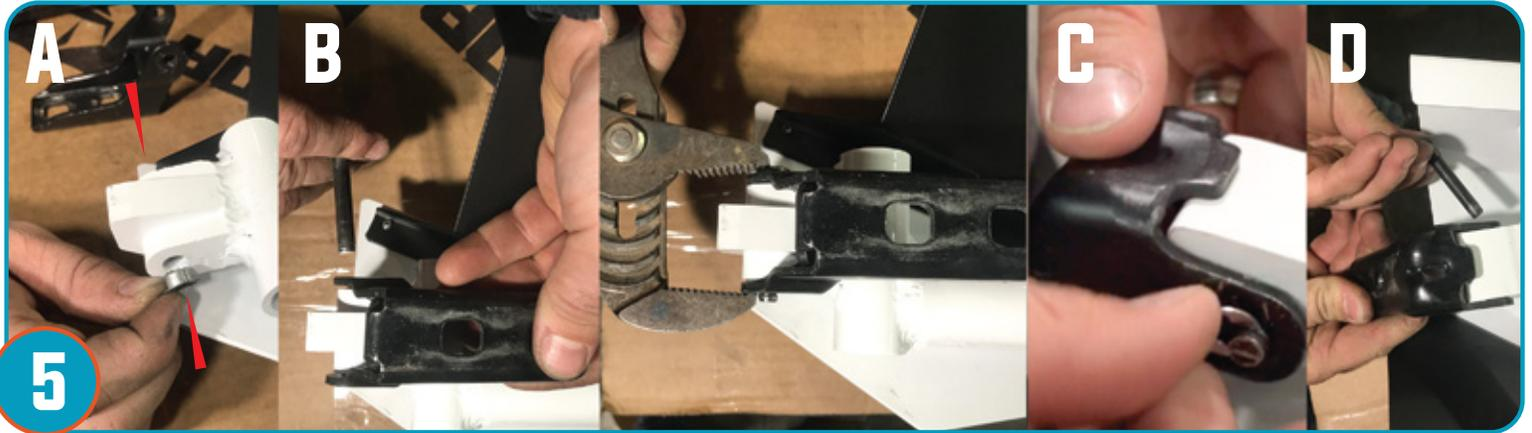
**5** A. Insert bushings removed from step 2 for top and bottom hinges of the Pro Armor door. B. With the inside of the door facing up, place stock hinge as shown in picture. Insert pin through lower hinge. Firmly squeeze door hinge to ensure pin is all the way through. C. Install C-clip on pin. D. Repeat for upper hinges. Repeat for opposite rear door.
