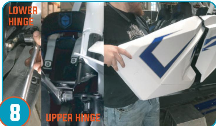
**8** Remove stock door by removing 4 bolts per door and remove lower & upper hinge to remove door from vehicle. Repeat for opposite door.
