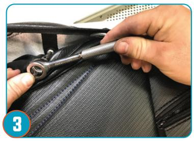
Using the Provided bolt secure the door bag to door lining to main zipper compartment as shown. Repeat for opposite door.
