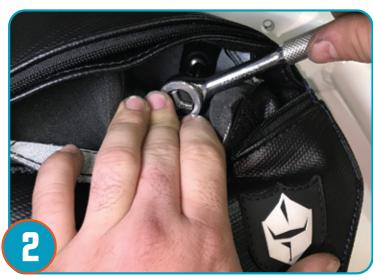
Using the Provided bolt place door bag in place and secure the door bag to front zipper door lining (1- bolt for each, inside zipper compartments) as shown. Repeat for opposite door.
