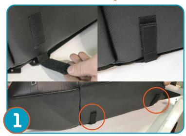
Run two door bag straps through door slots at locations shown. Then back up to door bag velcro, securing door bag to door.
