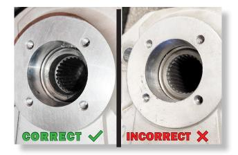
NOTE: On the portal boxes, the drive gear splines should be recessed to accommodate the shorter drive shaft splines.
