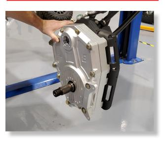
Apply water-resistant grease to the drive splines. Be sure to apply product all around the outer edge as well.
