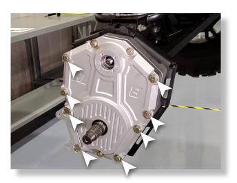
Loosely fasten all (8) bolts with 1/2" flat washers and 1/2" lock nuts. Ensure parts fit correctly then torque. (3/4) [105 ft lbs].
