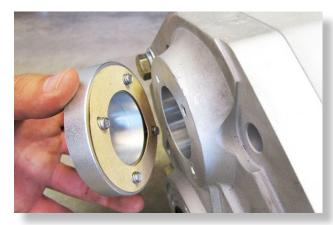
Remove the  $1/4-20 \times 3/4$ " screws & cap/gasket from the lid of the portal box.
