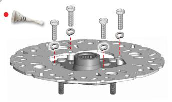
Install the rotor and secure it to the hub by applying LOCTITE (RED) to the (4)  $3/8 \times 1-1/4$ " hex head bolts & (4) 3/8 lock washer (7/32) [45 ft lbs].
