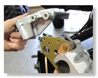
Remove the brake caliper mounting bolts (15mm). Remove the front mud scraper (8mm). KEEP ALL FACTORY HARDWARE. DO NOT REMOVE BRAKE LINE. Set caliper aside.
