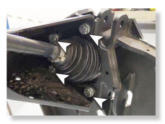
Install the backing plate to the trailing arm using M10 x 35mm bolts and 10mm flat washer on each side.
