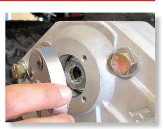
Align the portal box lid cap & gasket. Use the 1/4-20 x 3/4" screws and install the cap to the portal box. [8 ft lbs].
