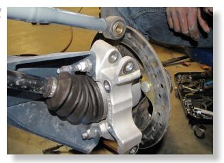
Remove the bolts and nuts that attach the rear knuckle to the UPPER & LOWER RADIUS BARS (15mm).
