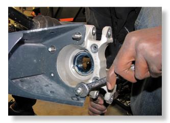
Remove the bolts and nuts that secure rear knuckle to the TRAILING ARM (15mm) Remove the rear knuckle.
