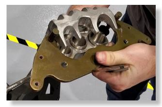
Remove the stock hanger bracket from the caliper.
