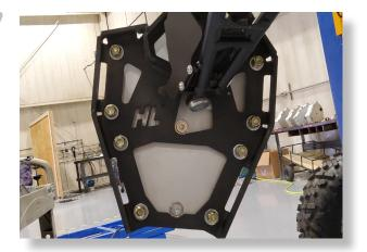
Insert the **bolts** through the corresponding **holes in the backing plate**.
