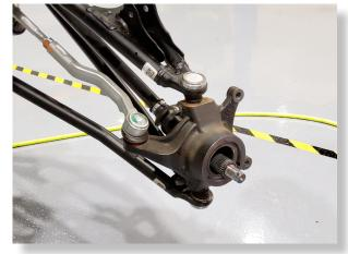
Remove the cotter pin, axle nut, and washers from the hub assembly, then remove the hub. (27mm)
