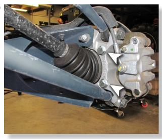
Remove the brake caliper mounting bolts from the hub assembly (15mm). Set Brake caliper aside.
