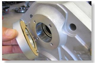
Remove the  $1/4-20 \times 3/4$ " screws, cap, and gasket from the lid of the assembled portal box.
