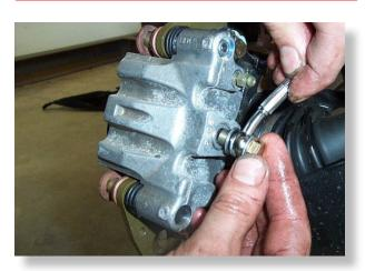
Disconnect the **rear factory brake lines** from the **calipers**. Have a container ready to collect brake fluid.
