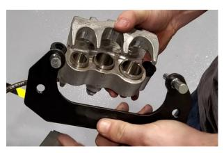
Install the supplied hanger bracket (108M) to the caliper. REINSTALL BRAKE PADS.
