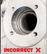
NOTE: On the FRONT & REAR portal boxes, the drive gear splines should be recessed to accommodate the shorter front drive shaft splines.
