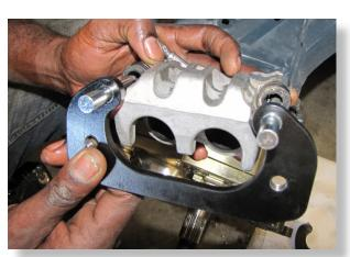
Remove the stock hanger bracket. Install the **85X hanger bracket** into the brake caliper.
