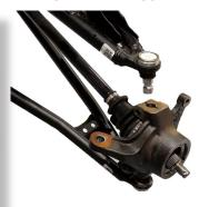
Disconnect the **Upper ball joint** by removing the **bolt** at the knuckle **(15mm)**.
