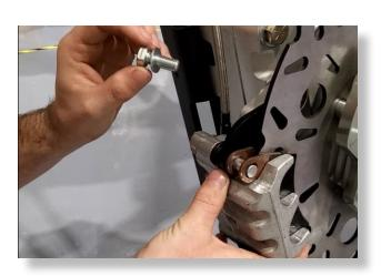
Reconnect the line and Install the caliper onto the portal box. Use the 10x25 bolts with 10 mm washer to secure the caliper to the bracket [30 ft lbs]. (These replace the factory 50mm bolts)
