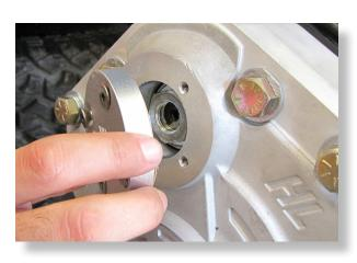
Align the portal box lid cap & gasket. Use the 1/4-20 x 3/4" screws and install the cap to the portal box [8 ft lbs].
