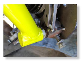
Use a 12mmx 65 bolt to secure a radius bar. Install a 12mm washer on each side and secure it with a 12mm lock nut. (18mm) [90 ft lbs].
