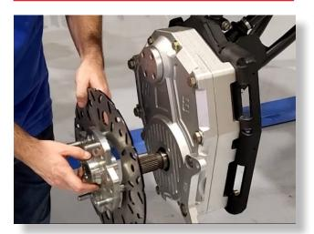
**Apply waterproof grease** to the spindle splines and slide the brake rotor onto the spindle shaft.
