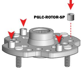
**Place the 1/2 spacers** over the tapped holes. These spacers go **BETWEEN** the hub and rotor.
