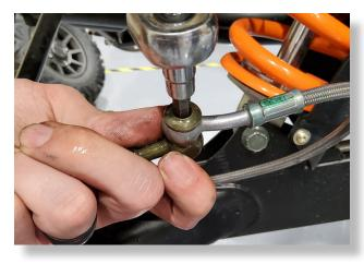
Disconnect the stock brake line from the caliper. Have a container ready to collect brake fluid. Locate the proper BRAKE LINE EXTENSION. Using the supplied button head hex drive banjo bolt, connect the STOCK BRAKE LINE to the BLIND-END BRAKE LINE EXTENSION. Ensure the copper washers are on each side of the banjo fitting.
