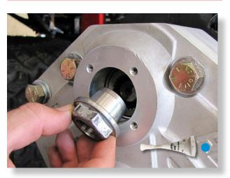
With the portal box installed, apply LOCTITE (BLUE) to the supplied M18 axle nut PGLC-AXNUT-4 and torque onto the drive shaft axle. (30mm) [20 ft lbs].
