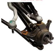
Disconnect the **tie rod** from the knuckle (**18mm**).
