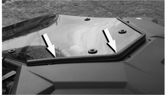
4. If you are using your roof with a windshield the 21" rubber gasket is provided to create a seal between the two parts. If not put in a safe place to use if and when you get a windshield. If needed install across the front of the roof as shown in the photo below.
