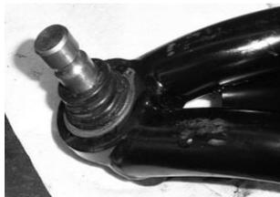
15. You will need to remove some material from the area where lower control arm mounts to the frame. You will only need to remove a small area nearest the axle boot.
