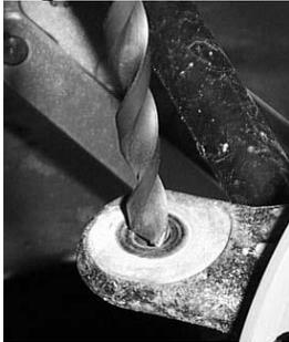
20. Once you have drilled the hole, use the 1/2 x 4" hex bolt and the two high alignment cones and connect the heim joint to the knuckle.
