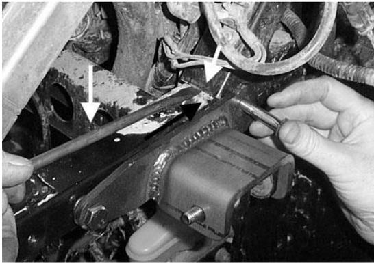
10. Insert the 10x95mm hex bolt through the shock mount bracket, shock eyelet, and spacer. Fasten it using the 10mm lock nut.
