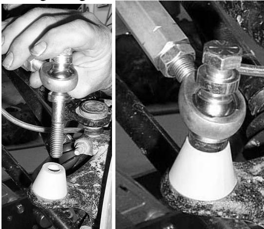
22. Place the 1/2" washer and 1/2" lock nut on the bolt and torque tight.
