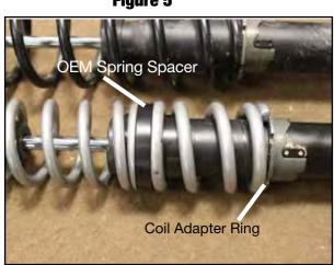
5. Make sure a coil adapter ring is installed on the end of the short spring contacting the preload adjuster ring as well as on the end of the long spring contacting the OEM retainer.
