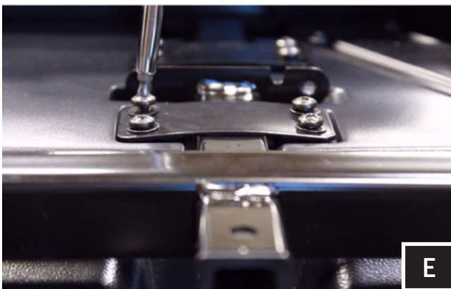
E. While applying pressure to keep the enclosure secure against the front wall, tighten the top brackets, as they tighten they will bend slightly to add pressure and avoid any vibration, now tighten the lower L bracket to the enclosure
