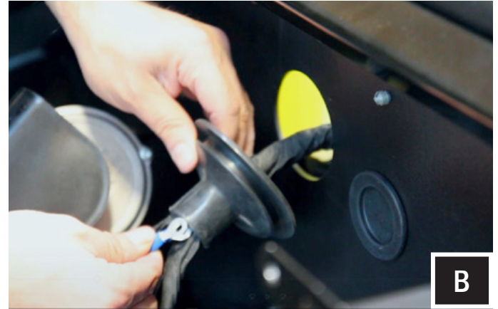
B. Pull the MRB3 POWER and GROUND wires through the rubber grommet and feed through the hole in the firewall to the power strip located on the opposite side of the firewall.
