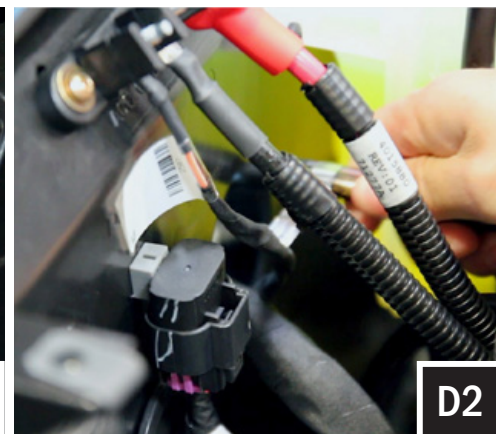
D. Feed the connector end of the Amp power wire through the center console to the other side of the firewall (D1). Then feed the power wire through the grommet hole (D2) and through the rubber grommet with the rest of the vehicle's wiring and cables (D3). Do the same for the 2nd Amp power & rear speaker wire.
