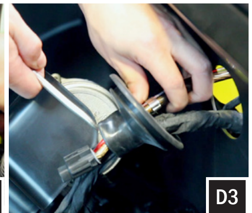
D. Feed the connector end of the Amp power wire through the center console to the other side of the firewall (D1). Then feed the power wire through the grommet hole (D2) and through the rubber grommet with the rest of the vehicle's wiring and cables (D3). Do the same for the 2nd Amp power & rear speaker wire.
