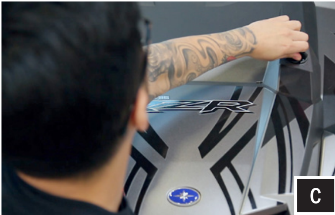
C. Remove hood by turning locking pins and lifting up.
