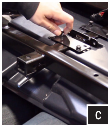
C. Lift the enclosure into place and align the top channel in the grab handle bar. While holding the enclosure in place, loosely attached the flat brackets to the top of the enclosure using the long screws provided.
