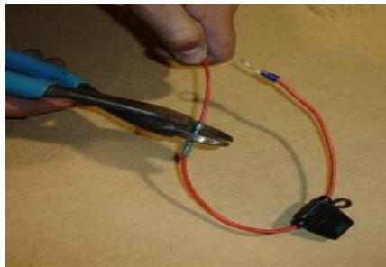
**12)** Crimp the supplied fuse holder onto the end of the RED wire and attach to the battery "+" terminal
