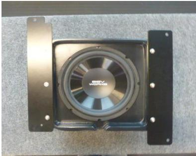
Using the 6 M6x1.0 screws and washers provided, attach the 2 brackets as shown
