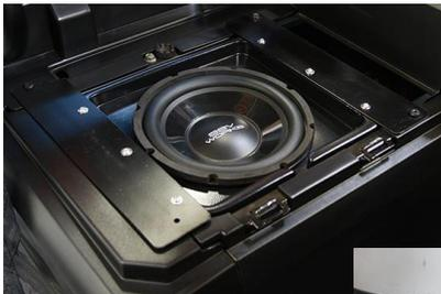
You can now place the enclosure in position under the seat and re-install the factory Torx Bolts, use the included "self-tapping" screw for the final hole location on the lower left bracket. Plug the input connector to the amp out connector from the overhead unit.
