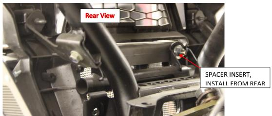
7.) MOUNT TO FRONT LOWER A-ARM BOLT. INSTALL BOLT FROM THE REAR.
