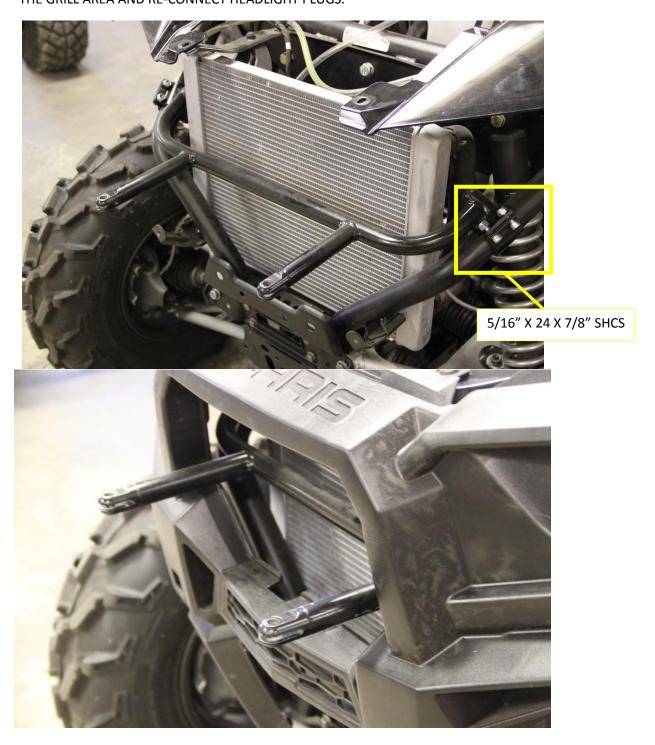
4.) TO USE GRILL INSERT WITH BUMPER, CUT OUT PORTION AS SHOWN ON THE SUPPLIED TEMPLATE.
